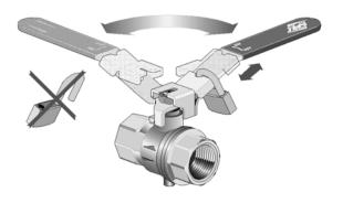
Lockable only in closed position when assembled on s.93 1/4":1" RuB range.
