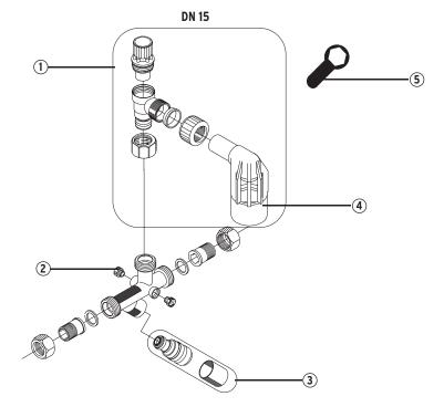
Exchangeable pressure relief valve 2115.1 6 bar 8 bar 10 bar
